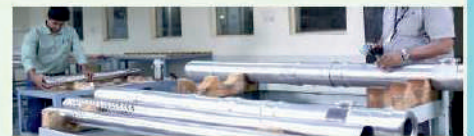
Coolant Channel Assemblies
